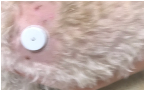
The sensor is glued to the dog's skin.
